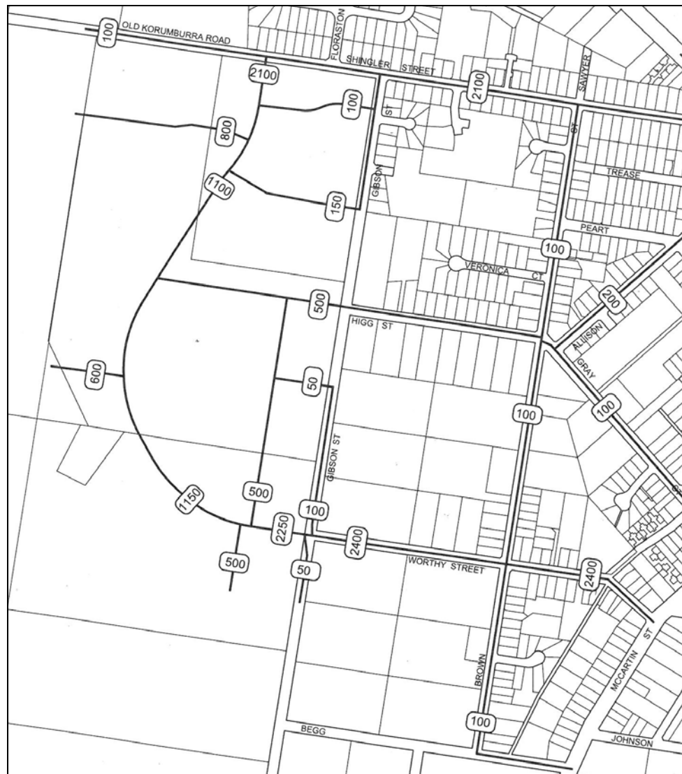
FIGURE 4 : ESTIMATED DAILY VEHICULAR TRAFFIC GENERATION
