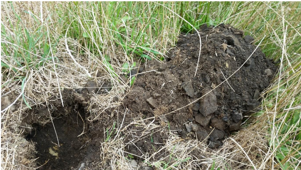
Photograph 4: Testpit samples taken along the former railway. Imported railway ballast and fill materials, including ash and coal, were present within all samples taken along the former railway embankment. This was used as the foundations of the railway's track and was found at depths greater than 0.5 meters. Refusal on rock prevented the determination of the exact depth of the railway ballast and fill material layer.
