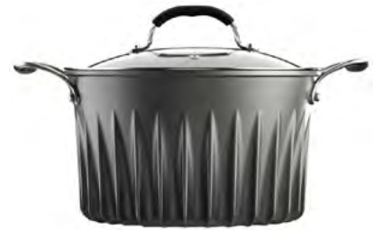
↑ The Flare Pan range from Lakeland in the UK feature fins to increase the surface area of the pot which improves heat absorption on a gas cooktop by up to 40%.
