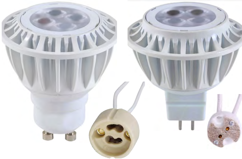
↑ These two downlight retrofit bulbs from Crompton Lighting look similar, but are quite different. The bulb on the left has a GU10 base and runs straight from mains voltage, so requires no transformer. The other bulb has a GU5.3 base (commonly referred to as an MR16 lamp) and requires 12 volts and hence the use of a transformer.
