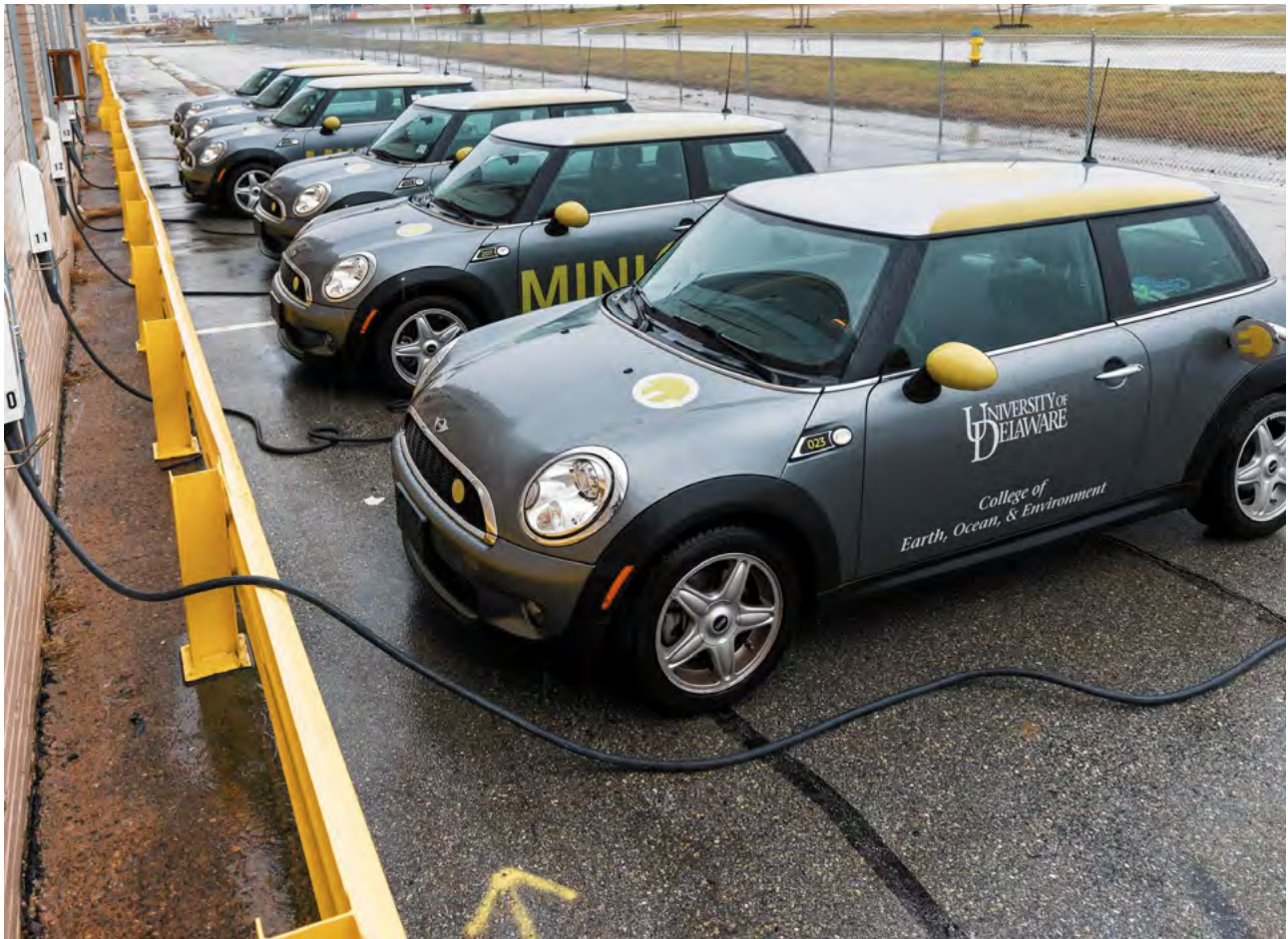
↑ The future is now...a fleet of Mini-Es being used by the University of Delaware to supply power back into the grid when it's needed most.
