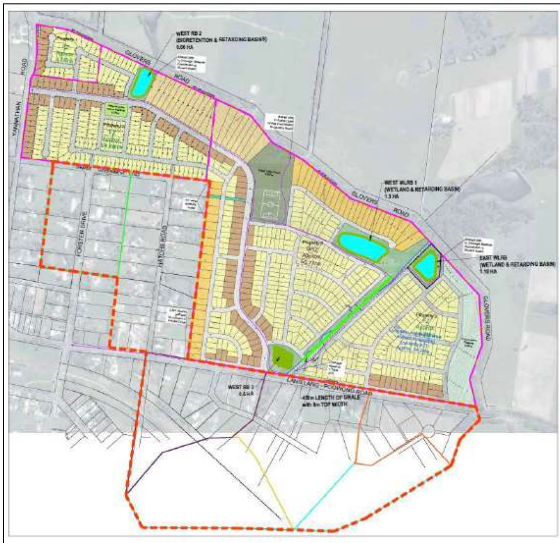
Figure 5: Post Development Catchment Plan Beveridge Williams Nyora Stormwater Management Strategy
