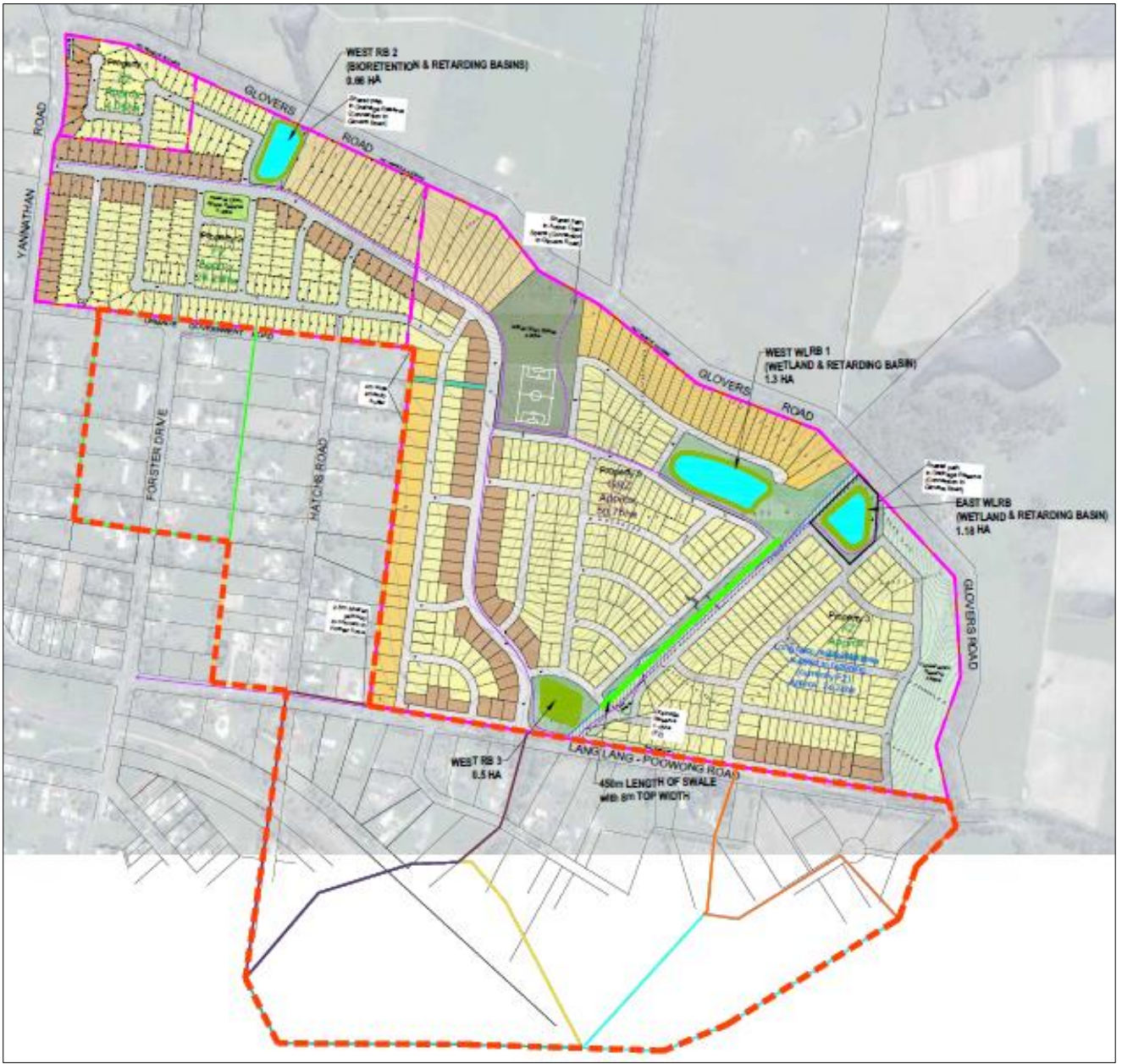
Figure 11: Concept Design Plan of the WSUD Assets (Not to Scale)
