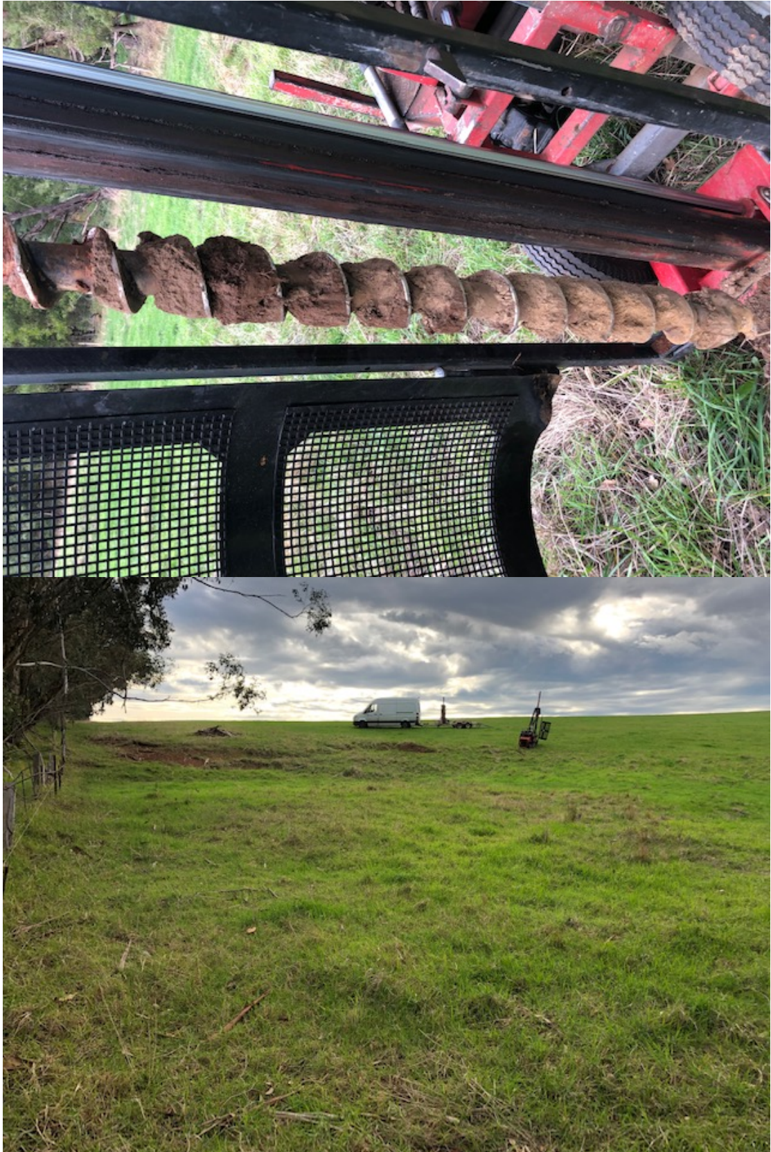
Plate 3 (Above) and Plate 4 (below) Inferred uncontrolled fill (28/5/19)
