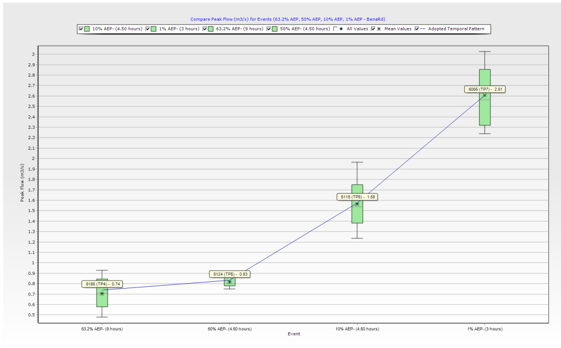
Figure 51. Estimated Bypass and Floodplain Flows
