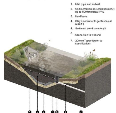
Figure 17: Typical Sediment Basin Profile
